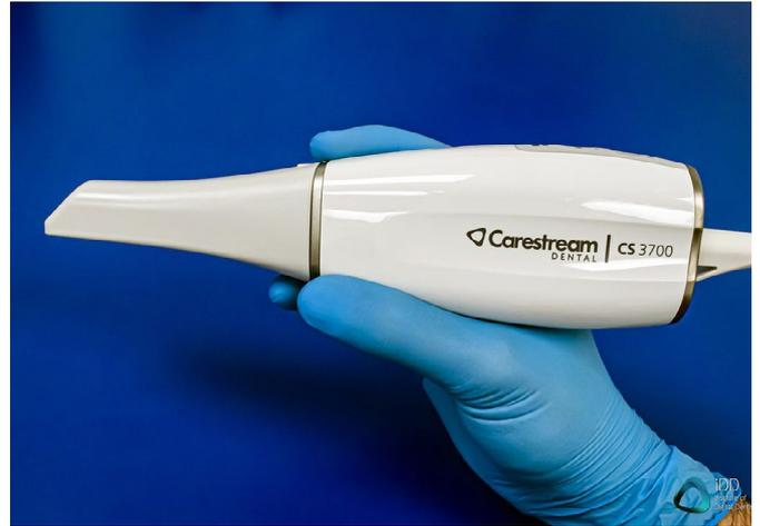
*CS3700 with the 'Side-Tip' scanner head attached and side-on hand position.*
