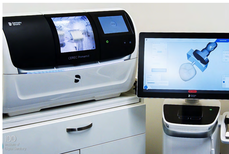
CEREC Primemill milling a restoration. You can see the blue LED stripe indicating milling progress.
