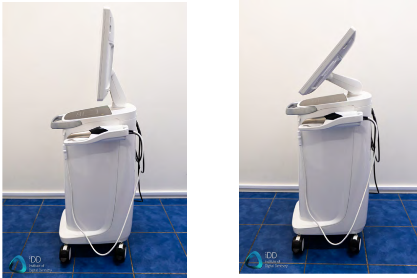
The CEREC Primescan monitor can be rotated as shown above
