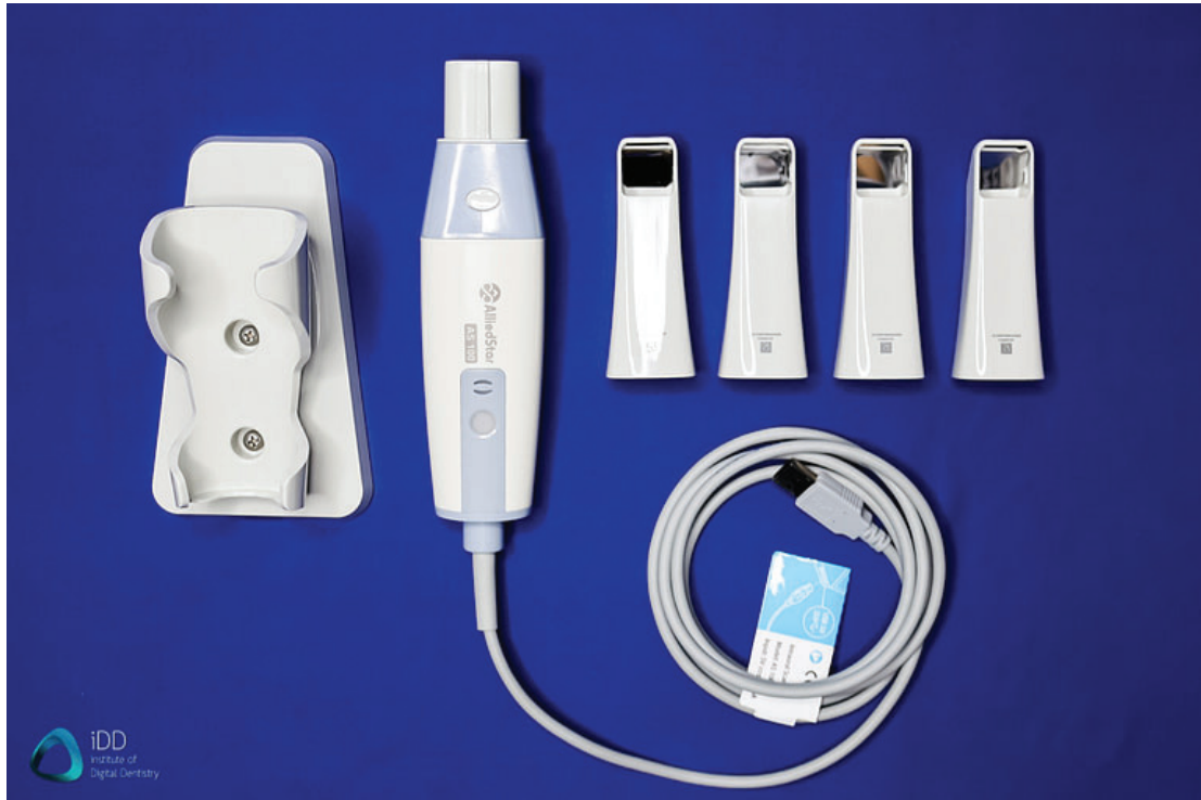
The Alliedstar AS 100 has one cable coming from it that connects to the computer via USB 3.0
