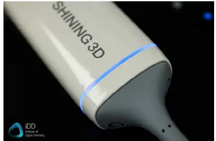
The LED ring shows you the scan and connection status.
