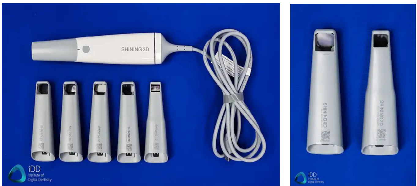
The Aoralscan 3 comes with 5 scanning tips. Adult and child sizes are shown.
