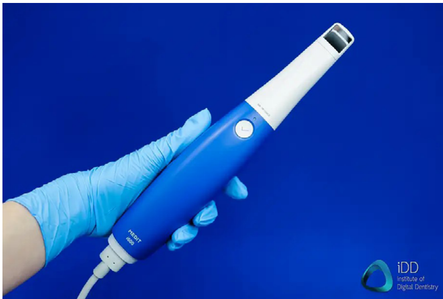
Medit i600 with scanning tip attached in reverse
