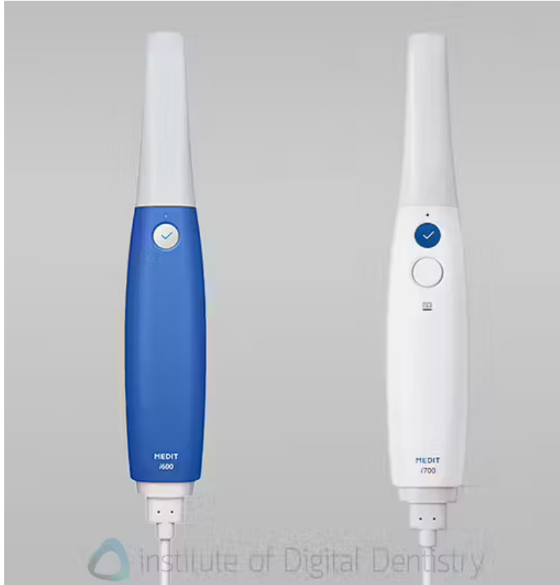
i600 next to the i700. Note the lack of a remote control button and UV indicator on the i600
