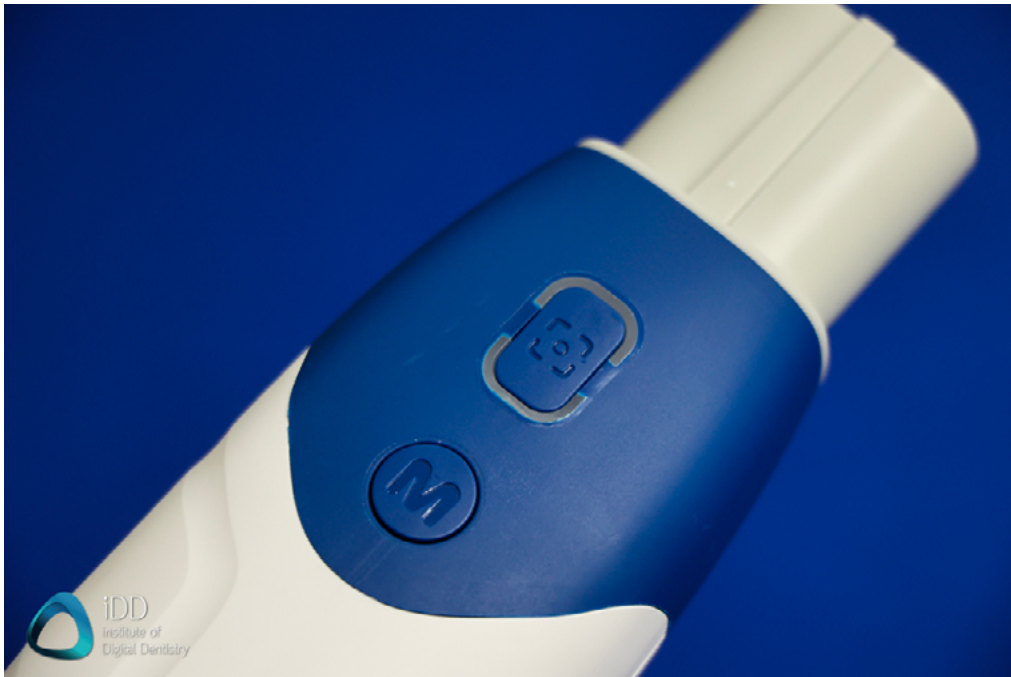
Scanner button on both sides. Mode button beneath the scanner button.
